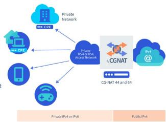
6WIND vCGNAT works on standard x86 and ARM servers to provide flexibility and costefficiency for small and large deployments.
