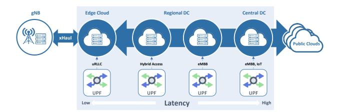
With its capability to create virtualized and isolated network instances, the 6WIND UPF provides a tailored foundation for implementing an efficient network slicing to support diverse use cases within a unified 5G infrastructure ranging from massive IoT deployments to ultra-reliable low-latency communications.
