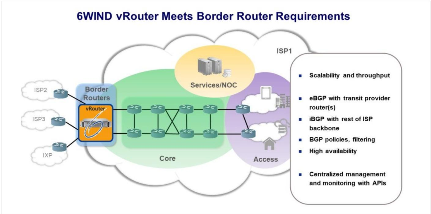
Figure 2. 6WIND border vRouter connects multiple ISP networks.<sup>2</sup>
