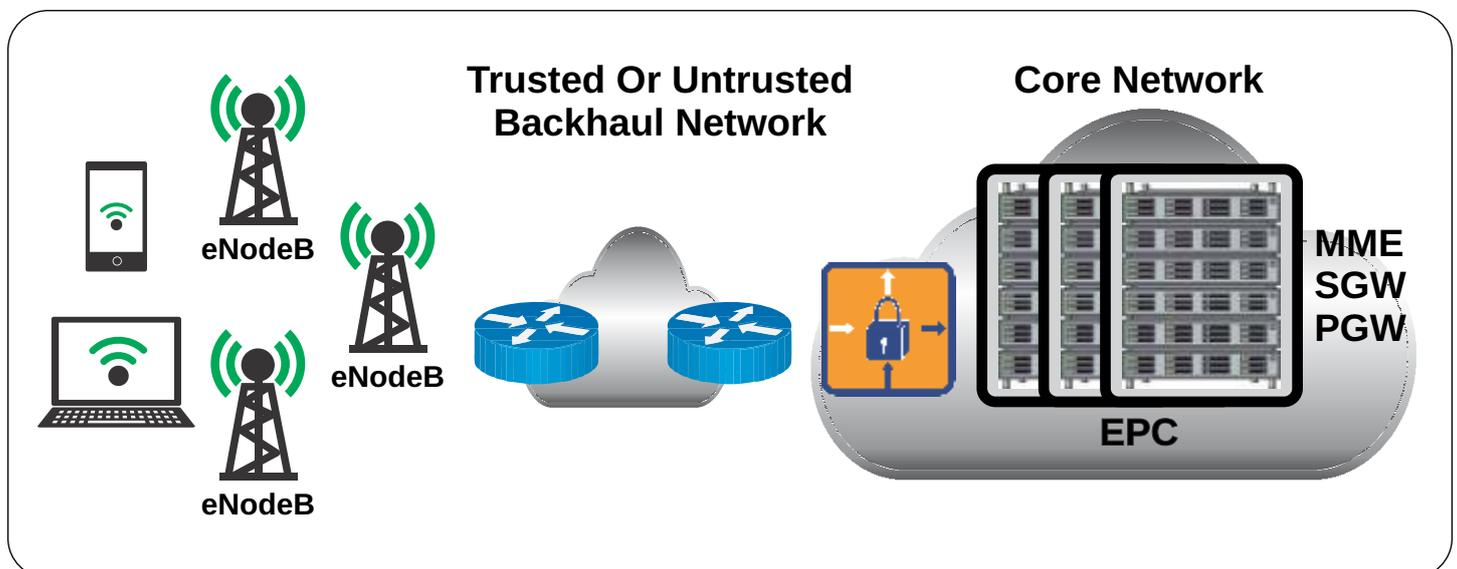
The main component of SAE is the EPC (Evolved Packet Core). EPC equipment has to manage a large number of subscribers via a Mobility Management Entity (MME) and process the aggregated traffic for 4G users via a Serving Gateway (SGW) and PDN Gateway (PGW). Compared to the previous generation of mobile networks, the combination of an increasing number of mobile users and per-user bandwidth led to critical performance and scalability challenges for LTE EPC.
